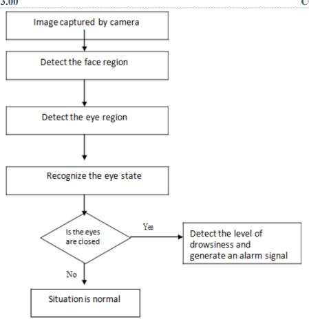
1. We first capture the face image of the driver using a web camera located inside the vehicle .
